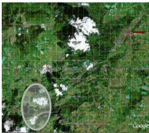
Figure 5.1. Typical satellite pixel in Europe with sizes of about 4x5 km 2 .
